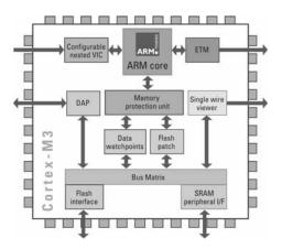
Figure 1: Block diagram of the Cortex-M3
